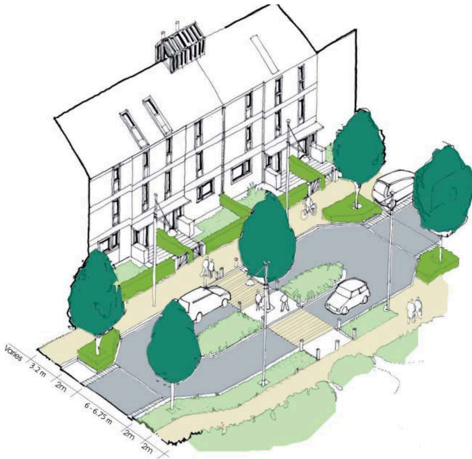
'The Avenue' - Axonometric of traffic calming measures
